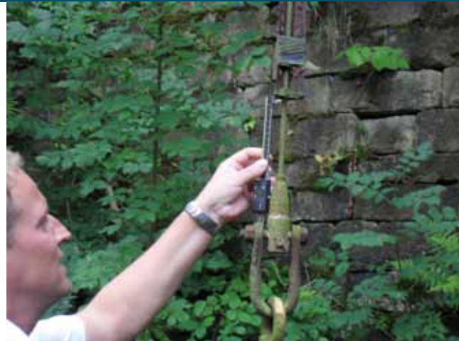
Tim Balderson, Business Development Director, Linear Composites, confirms total creep of only 0.23% in a Parafil® rope made with Kevlar® after 34 years continual load of 1200 kg (40% of NBL).
