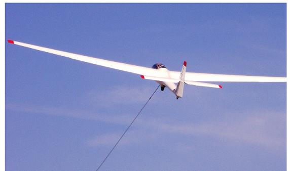
Parafil cable has been used by the club for more than 15 years. Each 600 metre length of PARAFIL® cable will normally survive being dragged over the very abrasive surface of the runways for some 800-900 launches, approximately 8 to 9 months of use, before having to be scrapped.
