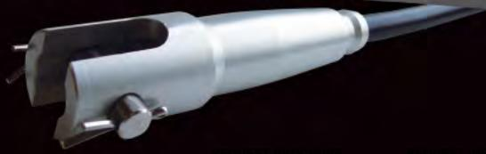
PARAFIL® ropes consist of a core of closely packed, high strength aramid, PBO or high tenacity polyester fibres, lying parallel to each other, encased in a protective polymeric sheath. This structure is combined with a specially designed termination technique.
